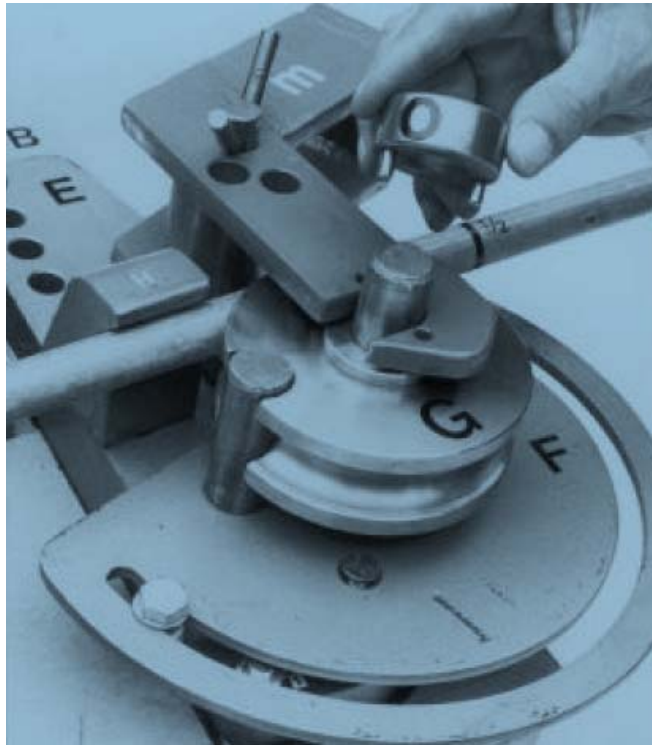
Fix ring O over the spindle and lock it up with the 2 doweled joints
