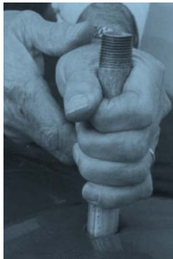
The thread-end of the pipe must be kept outside of the drum. All pipes stand perpendicular of the drum
