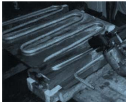
Take the burning soldering lamp and move it slowly to and for alongside the triangle
