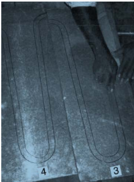
Sand the marked area in between the lines
