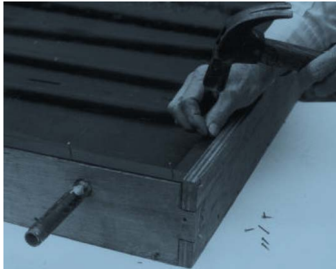
Fasten rubber strips over the rebates of sides A-B-C and D
